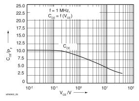
Figure 5. Transistor Capacitances (typ.)
