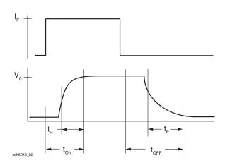
Figure 2. Switching Waveform
