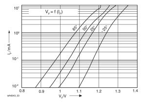
Figure 3. LED Current vs. LED Voltage
