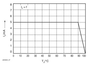
Figure 7. Permissible Forward Current Diode
