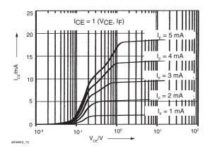
Figure 10. Transistor Output Characteristics
