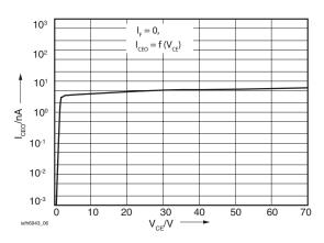
Figure 6. Collector-Emitter Leakage Current (typ.)
